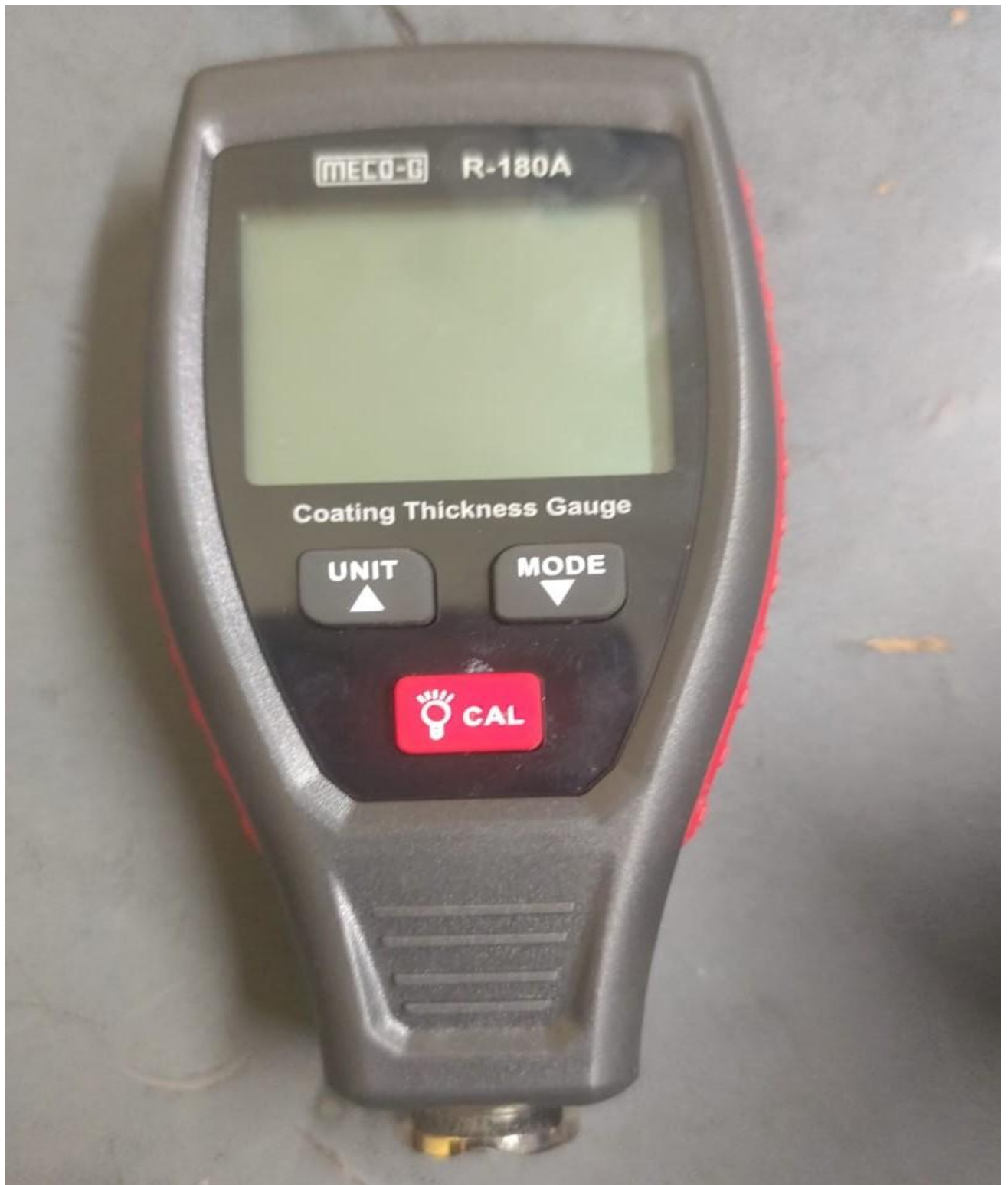
ELCOMETER (PAINT COATING THICKNESS GAUGE)
